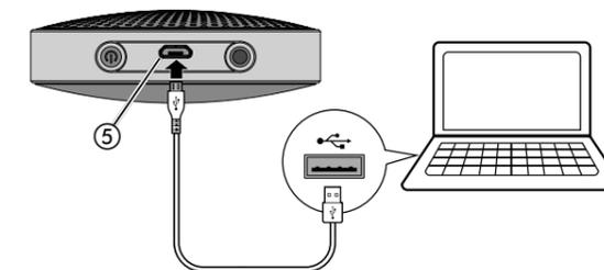
The rechargeable battery in your BAMSTER XS is charged via the USB cable. Charge it for approx. 3 hrs before first use.
