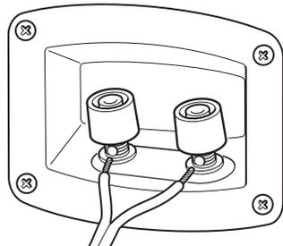
A connector terminal with two terminals is located on the back of each speaker; the speaker cable must be attached to them.
