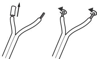
3. Split the single wire down by approx. 30 mm on both ends and remove approx. 10 mm of insulation each.
