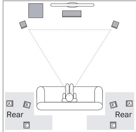
The rear speakers are set up or hung to the side of or behind the listener at a height of 1.20 m to 2.10 m (see the grey areas in the graphic).
