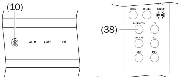
3. If the ULTIMA 40 ACTIVE NG is not connected to an external player, pairing will start automatically: The notice “Pairing” will appear on the display panel **(8)** and the button **(10)** will flash blue. Otherwise, push the button **(10)** or **BLUETOOTH (38)** and hold it down for approx. 2 seconds to start pairing. Pairing will be active for approx. 60 seconds.
