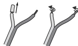
4. Turn the connector terminal counterclockwise until loose. Run the stripped cable end into the now visible hole. Close the terminal by turning it counterclockwise. The cable has now been clamped in place.
